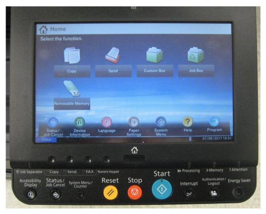
Up to 50 scan jobs can be saved as job programs within the scan menu or even on the Home screen to streamline workflow of commonly run jobs.
